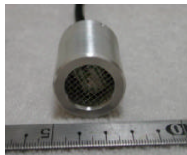
Fig.2 QCM sensor head. Size is 30mm (Diameter) and 45mm long (Typical Head)
